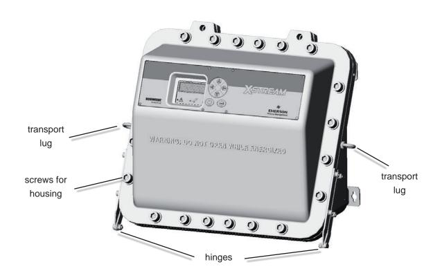
Fig. 1-11: X-STREAM X2FD - Front View
